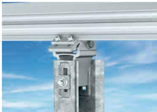
The toothed oblong hole allows height adjustment and takes up higher loads through a self-locking effect.
